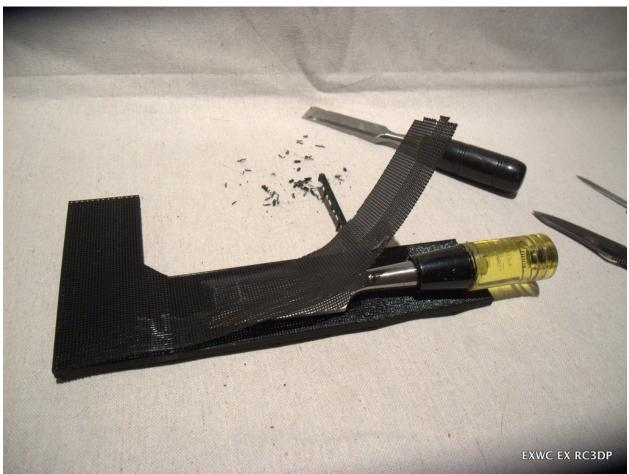
Figure 7: The first printed pier section required extensive deburring due to the support layer printed beneath the entire part.
