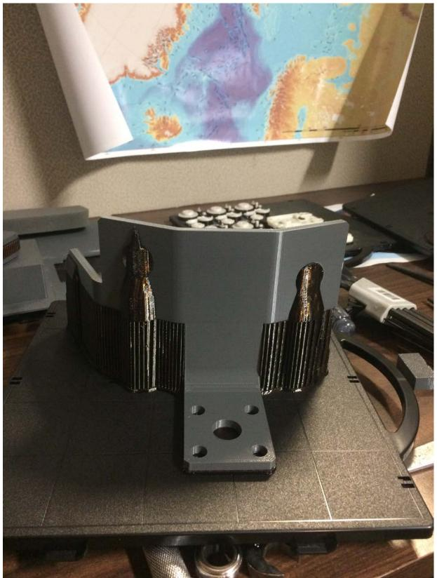
Figure 30: The fire extinguisher bracket was successfully printed on the Dimension 1200es. Note the multiple materials and disposable build-plate.
