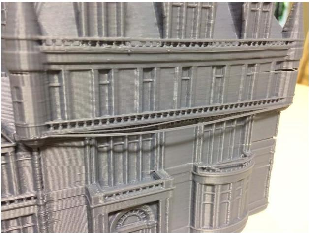
Figure 37: This surface detail of Vanderbilt mansion print shows unsuccessful elements of the print due to lack of support material.
