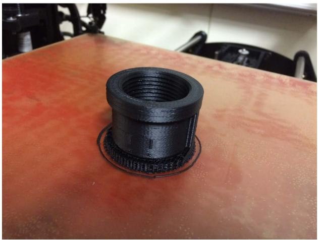
Figure 39: This pipe end cap was downloaded as a model file from McMaster Carr, and printed in ABS plastic on the TAZ5.
