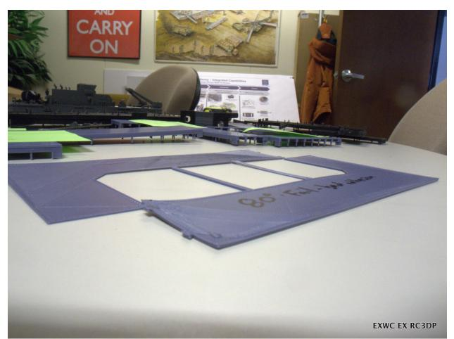
Figure 21: Attempts to print HIPS parts at reduced bed temperatures resulted in adhesion failures.
