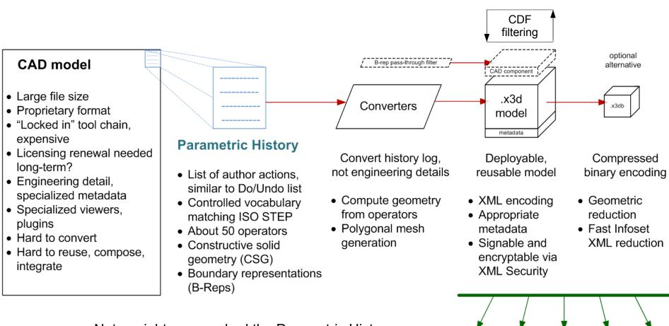
Note: might even embed the Parametric History file as metadata in .x3d model, in order to enable reasonably accurate round-trip regeneration of the original CAD model despite data lossiness.
