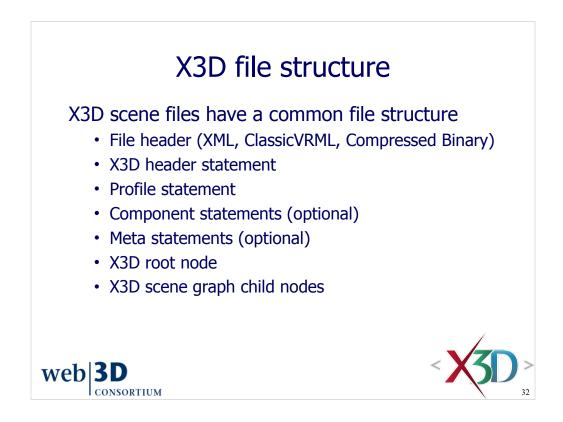
The X3D scene root node is implicit in ClassicVRML encoding and not listed per se.
