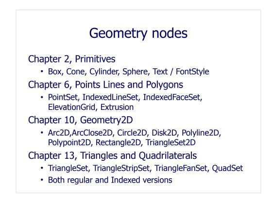
The principle that one geometry node goes inside each Shape, and next to each Appearance, is consistent for all the different geometry nodes available in X3D.
