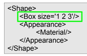
Shape must be parent node, can only hold one geometry node Appearance and Material nodes define colors, transparency, etc.
