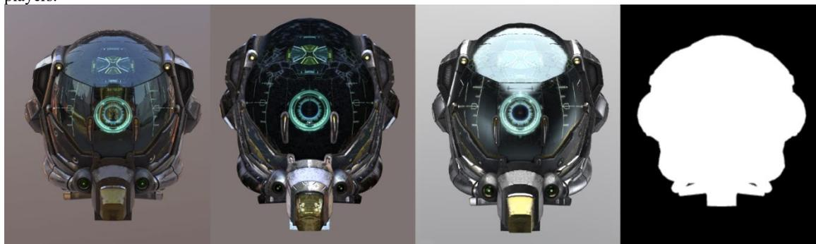
Figure 3: Comparison of a single model rendered (a) natively as glTF in glTF Sample Viewer, then converted to X3D in (b) view3Dscene, (c) X3DOM, and (d) X\_ITE players.
